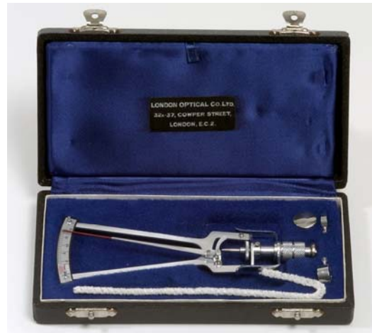
Figure 1 Schiøtz Tonometer. Photograph kindly supplied by The British Optical Association Museum, © College of Optometrists.
